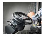
**Ergonomic steering wheel** It's adjustable and can also be tilted to the side. This decreases stress on the operator during driving and reversing.
