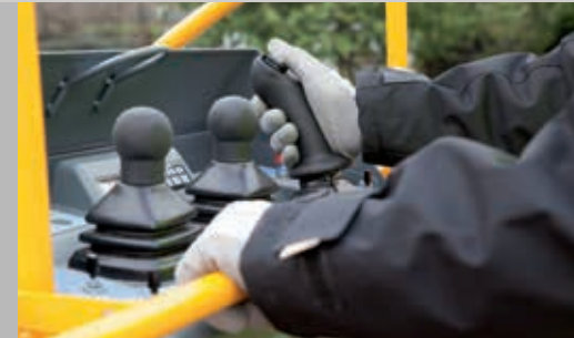
When driving, the joystick can be operated with only one hand, so the other can hold the safety rail
