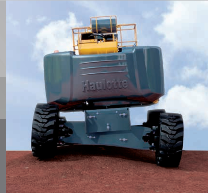
On the RTJ 0 and RTJ PRO models, the oscillating axle allows the 4 wheels to maintain contact with the ground at all times
