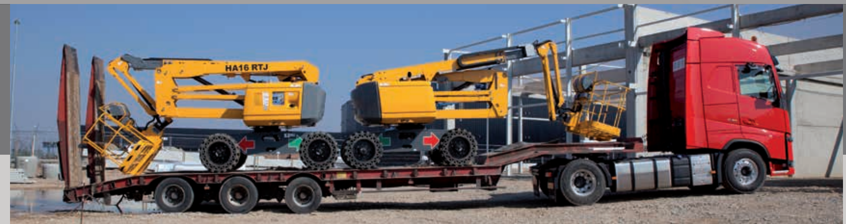
Economic transportation: thanks to the ability to fold the jib under the boom, one truck = 2 HA16 RTJ
