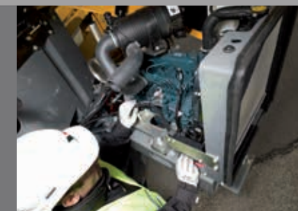
Swing out engine tray enabling direct access to key components
