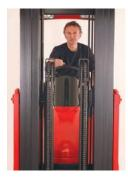
Flexi's famous "clear vision" triplex mast design, heavy duty German cold rolled 'I-beam' sections format. Integrated heavy duty side shift fork carriage is standard.
