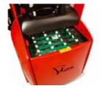
Low lift off or roll off for fast changes. Clear battery access with no components or motors underneath.
